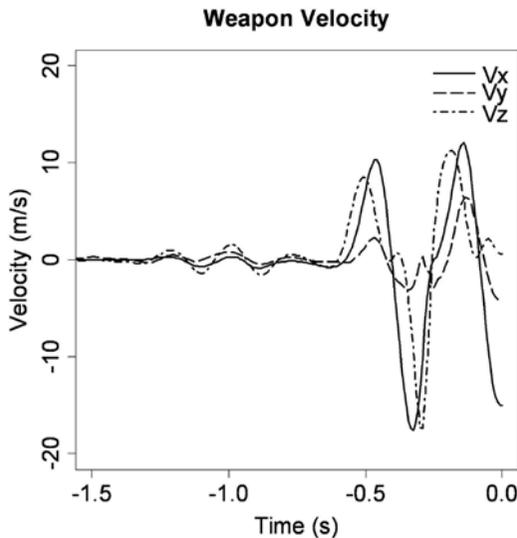
**Figure 5** — Weapon velocity. This figure shows the velocities of weapons X, Y and Z during the coupling and decoupling phase. The beginning of the decoupling phase is clearly identified by a velocity threshold on the Z axis. Time 0 corresponds to the moment of attack.
