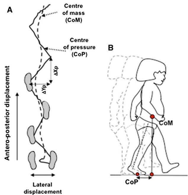
**Fig. 1** a CoP and CoM oscillation during a sequence of six steps. *Solid line* gives the CoP displacement, and *dotted line* gives the CoM displacement.  $\Delta Y_p$  = step width,  $\Delta X_p$  = step length. **b** Relative positions of CoM and CoP at the end of the single-support phase
